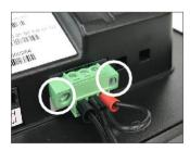
2. Then connect the adapter to a power source.
