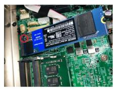
3. Insert and fasten the screw into the standoff.
