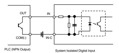
Note that the input's (IN-C) first and last pins are for VCC.
