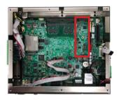
2. Insert the M.2 module into the socket by aligning the notch on the module with the small slot on the M.2 socket.
