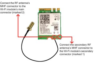
6. Plug the Wi-Fi module to the socket's connector by a slanted angle. Fully plug the module, and note that the notch on the wireless module should meet the break of the connector, then fasten the screw.
