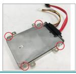
4. Connect the SATA interface and power cables to the SATA & power connectors on the main board.
