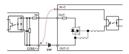
Note that the output's (OUT-C) first and last pins are for GND.
