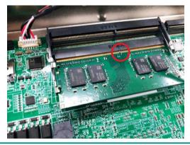
3. Slide the module into place. Once the memory module is fully inserted into the socket, press down on the top edge of the device to latch it into place.
