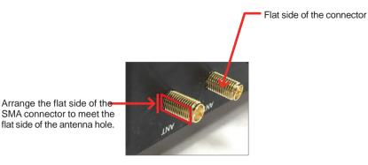
10. Mount the washer first and then the nut to the SMA connector. Make sure the nut is tightened.
