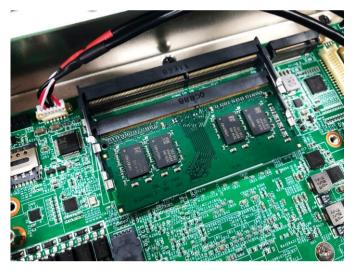
4. This way it's flat to the laptop's bottom. The carrier should snap into place with latches.
